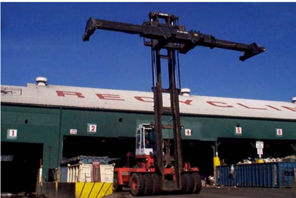
Installed on a 100,000 lb Lift Truck for Rabanco Recycling in Seattle, Washington.
